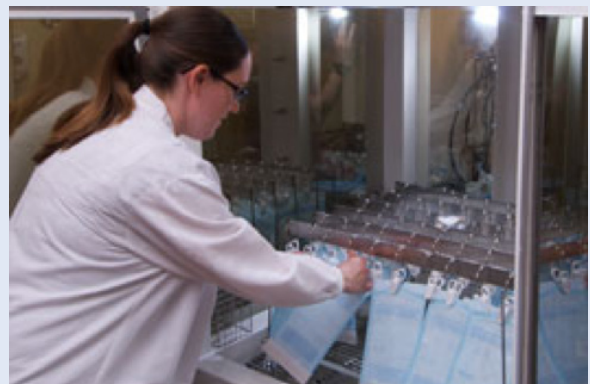
Figure 3. Chamber being filled with sample bags before exposure to the aerosol containing Bacillus spores.
